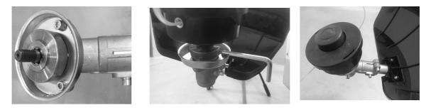
To remove the cutting head, put a locking tool in the hole of the shaft. Then unscrew the cutting head. This will have to be done tool off and cooled.
